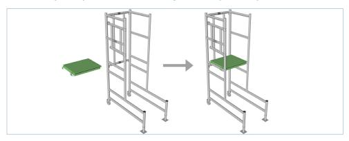
4. Place the detachable Ladder in position, and lock the bottom braces into place. Ensure the hooks are in place and locked. Then follow the same step with the top of the ladder
