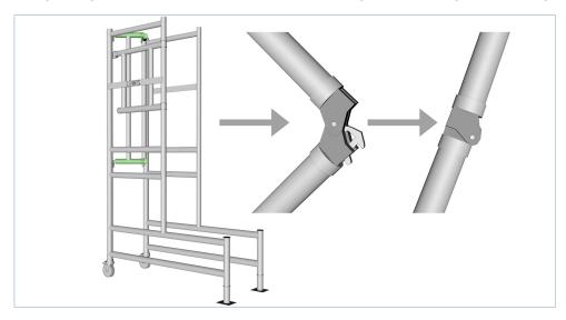
3. Place the podium platform at the chosen height, and safely lock into place the wind locks
